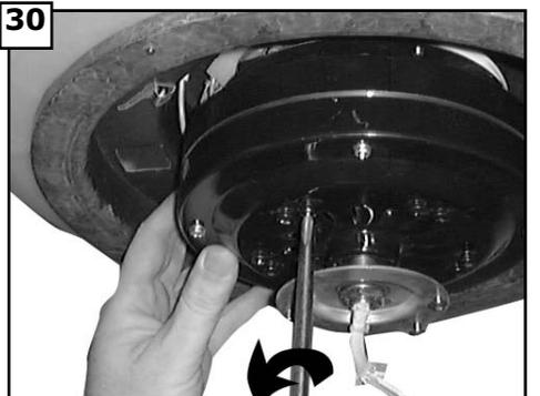
30 Remove motor screws from fan motor and save.
